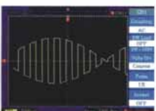
PSK PSK mode adjustable parameter: ( Phase 1, Phase 2, PSK time Trigger mode )
