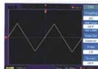
Triangle Wave - 2V, 10kHz Amplitude: 100 \mu Vpp ~ 20Vpp (High impedance) Frequency: 100 \mu Hz ~ 100kHz
